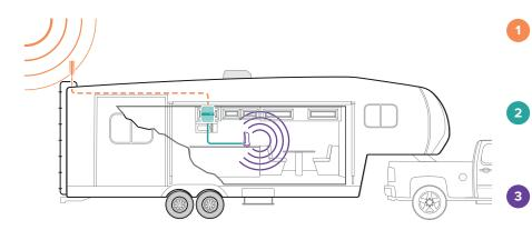
Receives signal: The powerful antenna reaches out to access a voice and data signal, and delivers it to the booster.
